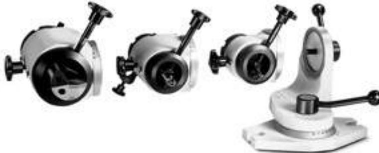
Using **botek grinding fixtures**, single flute gundrills can be reground on any good tool grinding machine. Depending on tool diameter, botek grinding fixtures are available as Model ZS (see illustration left) or Model PS (for solid carbide gundrills).
