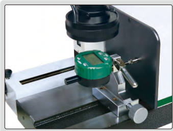
check digital indicators (detect digits on screen)
