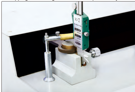
lapping measuring surfaces of caliper lower jaws
