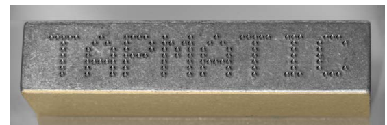
Point to point programming for creating characters with defined dot position or 2D Data Matrix codes.
